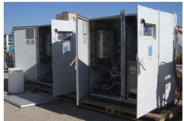
Figure 12. Two used Proton Onsite model H6m electrolysis plants are owned by AASI, stored in Golden, CO, and will be dedicated to the project.
