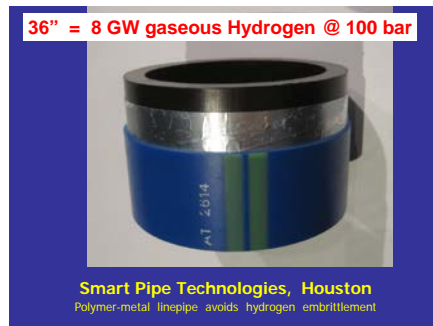
Figure 5. Transmission and distribution pipe: a thin Al or Cu foil provides the hydrogen permeation barrier, avoiding the hydrogen embrittlement danger inherent in steel linepipe. Hydrogen transmission pipelines are comparable in capex, and lower in O&M cost, than electricity transmission lines.
